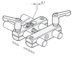
Line scaling on adjusting wheel for adjustment in 1/10 mm increments
